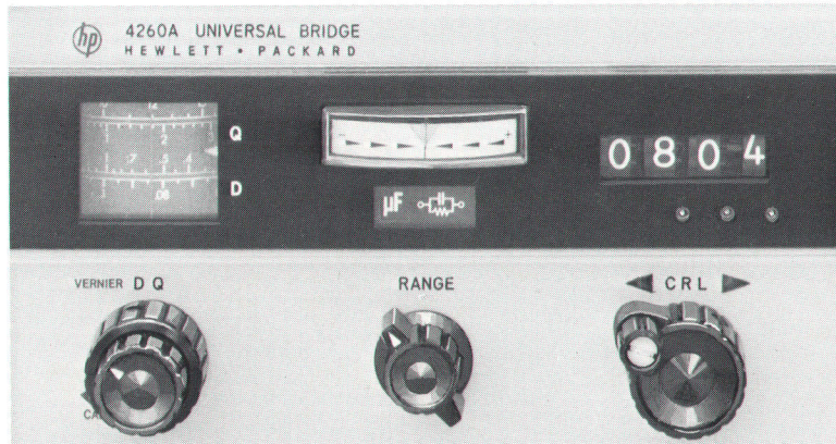
Fig. 4. Photo shows operating features which contribute to easier bridge operation. Readout is digital and decimal point is placed automatically by RANGE switch. Window above RANGE switch shows unit of measurement for selected range and functions; circuit diagram shows whether lossy component of reactance is measured as resistance in parallel with or in series with reactance. In 'Auto' mode measurements of capacitance and inductance, illuminated arrows above CRL control indicate direction that RANGE and CRL controls should be turned to achieve null.
